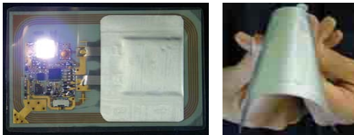
Fig. 2. Proto-type of the thin and flexible radical battery (NEC Co.) loaded on flash devices and smart cards.
